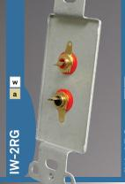
2 Gold-Plated RCA Jacks. Will install in standard "J" box. Wiring should be RG-59U or similar shielded coax.
