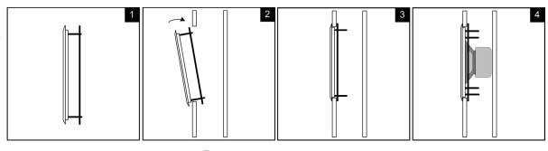
the speaker location on the wall. The RIB-LCR brackets are available from the distributor or dealer where the speakers were purchased. When the brackets are used the holes are cut when the drywall is installed. The cable can be tied off on the bracket after securing the cable to a nearby joist.
