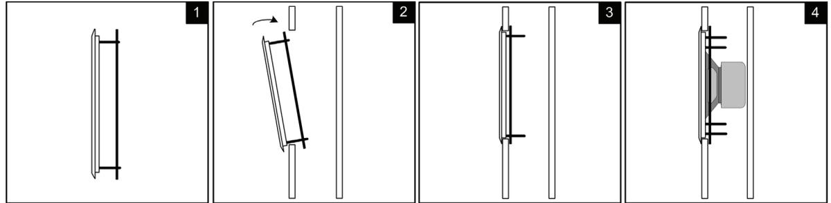
As the diagrams show, the speakers utilize a metal Retro Ring which, after tightening with the 4 screws provided, acts as a clamp to hold the magnet frame in place. **Note: Use only the 4 outer holes for mounting the frame.**
