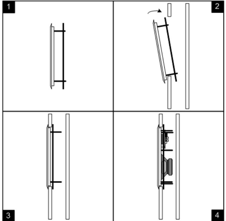
The more-closely spaced holes are toward the top. The frame should fit cleanly, without interference, in the cut-out hole. If the hole is a little small then trim the hole as needed. Lightly tighten the screws to secure the retro ring against the back of the wall (**see fig. 3**). Use care not to over-tighten the screws or the frame may become distorted.
