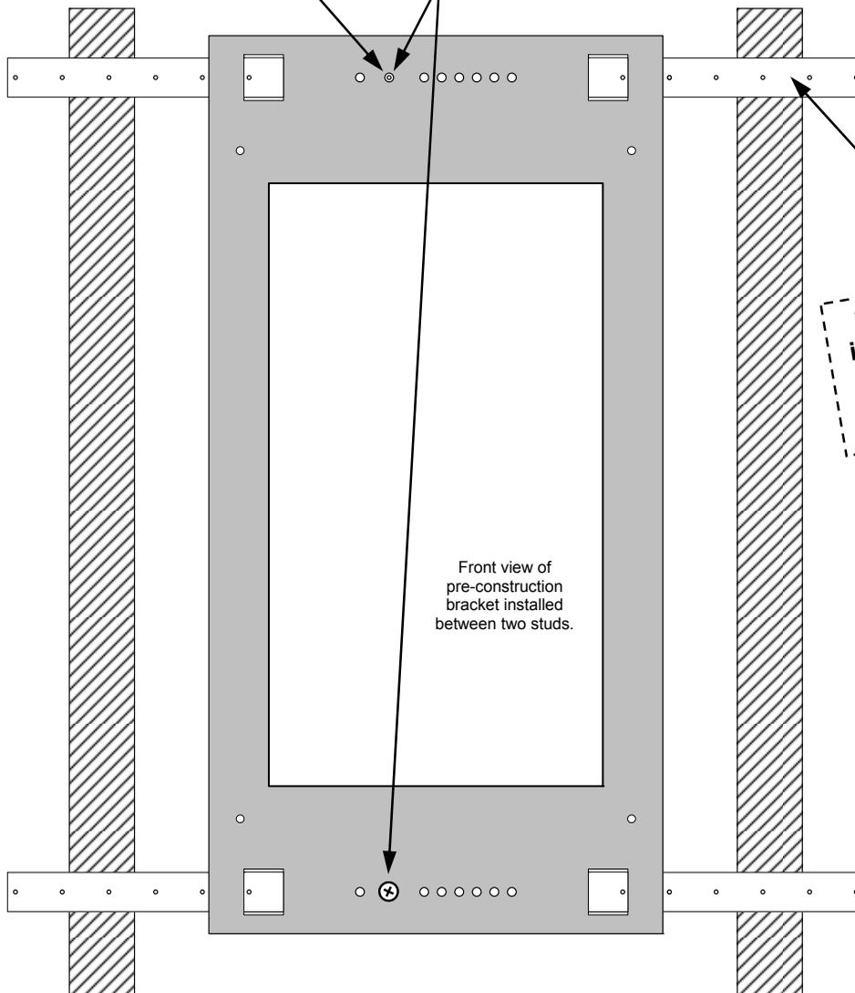
**Be certain to use a LEVEL when installing rectangular brackets on walls or the final installation will most likely suffer!**
