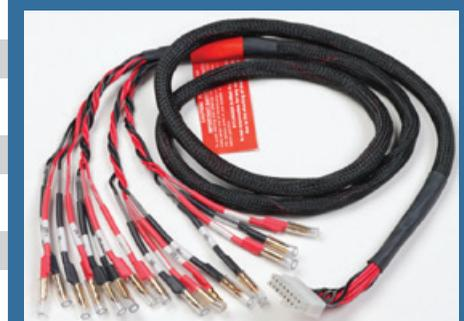
Each MB-4 provides connections for 4 pairs of speakers. The MB-4 wiring harness is approximately 4' in length. It is terminated on one end with a 16 conductor molded nylon locking connector and 16 high-grade gold plated banana plugs on the other end. The nylon connector snaps and locks into the rear panel of the SLX-4. These connections are not subject to "working loose" or becoming loose from minor movement.
